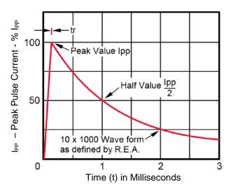
FIGURE 2 1<u>0/1000 µs Current Impulse Waveform</u>
