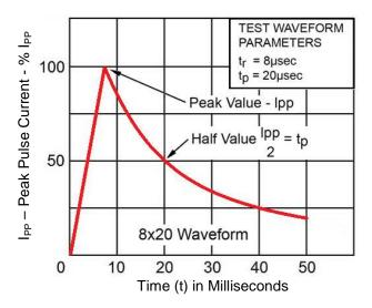
FIGURE 3 8/20 µs Current Impulse Waveform
